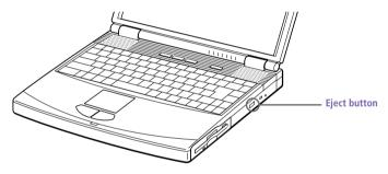
Place a DVD-ROM/CD-ROM in the tray with the label side facing up. For DVD-ROMs, which can be played on both sides, the side of the disc facing up is the side that plays. Push the disc onto the hub until the disc clicks into place.
